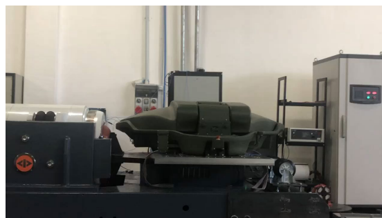
Figure 25 PDA-150-MIL Antenna System During Vibration Test (Actual Footage)
