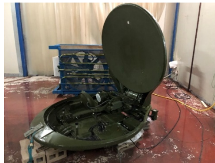
Figure 21 PDA-150-MIL Antenna System During Rain Test (Actual Footage)
