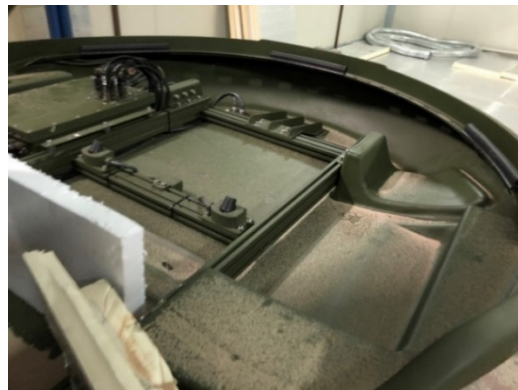
Figure 26 PDA-150-MIL Antenna System During Sand/Dust Test (Actual Footage)
