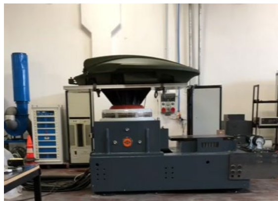
Figure 24 PDA-150-MIL Antenna System During Shock Test (Actual Footage)
