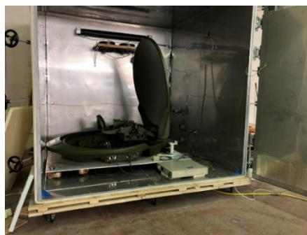
Figure 22 PDA-150-MIL Antenna System During Humidity Test (Actual Footage)
