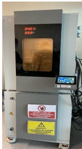
Figure 19 PFA-370-MIL Antenna System During Humidity Test (Actual Footage)
