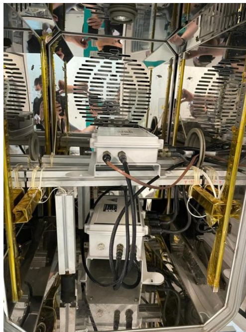
Figure 17 PFA-370-MIL Outdoor Unit And De-ice Controller Inside Temperature Test Chamber
