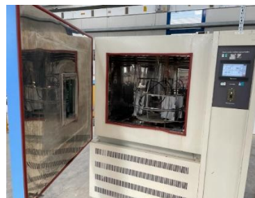
Figure 20 PFA-370-MIL Outdoor Unit And De-ice Controller Inside Solar Radiation Test Chamber
