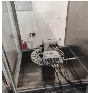
Figure 18 PFA-370-MIL Outdoor Unit And De-ice Controller Inside Rain Test Chamber
